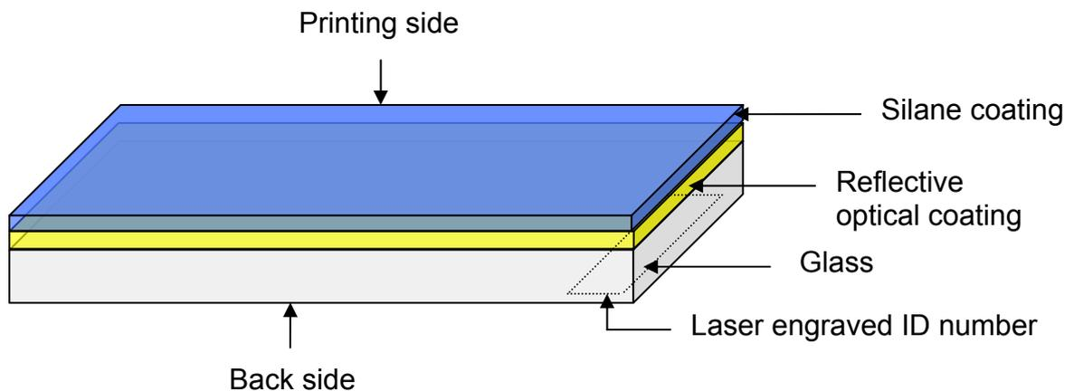
*Scheme of AmpliSlide™ functionalized substrate.*
